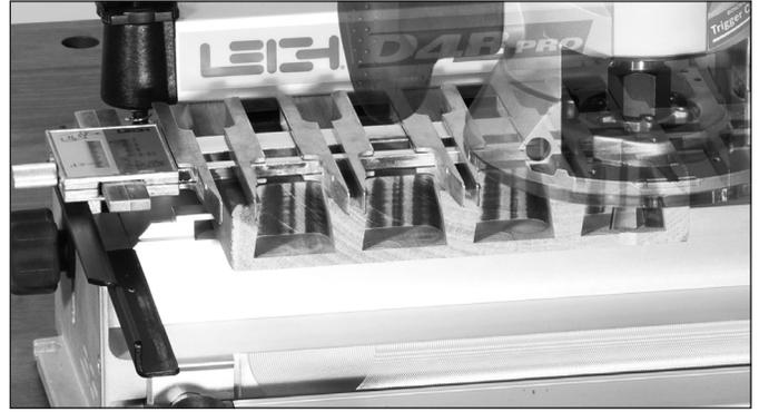
**14** Then, proceed to rout the pin board with the dovetail bit set at the correct depth. Remove the pin board and test the joint for fit. See sections 15, 16, 17 & 18 for fit and flushness adjustments.
