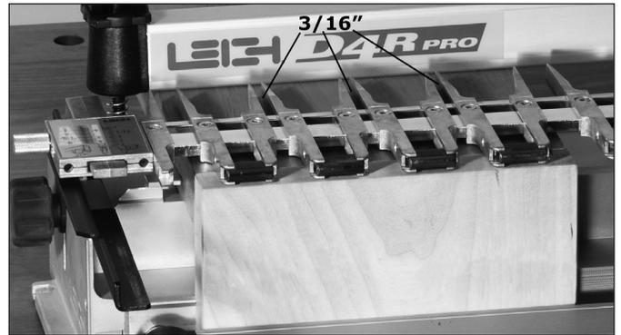
**4** Arrange the fingers in the desired joint pattern being sure to allow for a half pin at each edge of the board. **Note:** Finger pairs must be separated by at least 3/16" [4,75mm] to allow the e10 or 716TP guide bush to pass through.
