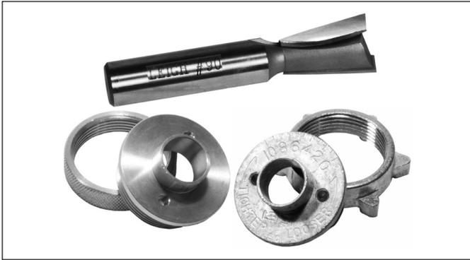
**1** Use the No. 90 dovetail bit with the e10 guidebush or the 716TP 5/8" [15,9mm] guidebush. The e10 guide bush set on the 5 mark will give a 1" [25,4mm] depth of cut. The 716TP will give a 15/16" [23,8mm] depth. Choose the combination that best suits your project. Trial and error will produce actual cutting depths.
