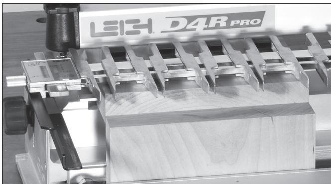
**11** Flip the finger assembly to the Half-blind Pin mode.
