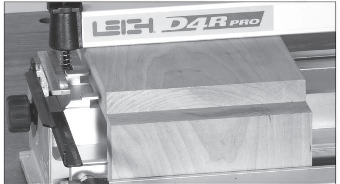
**10** Mount a pin board horizontally under the top clamp bar and bring it forward butting up against a scrap board mounted in the front of the jig.
