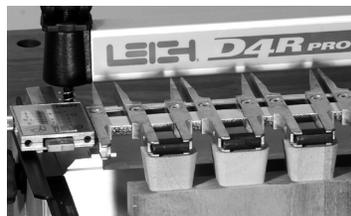
**Pins:** Flip the finger assembly to the Half-blind Pin mode.
