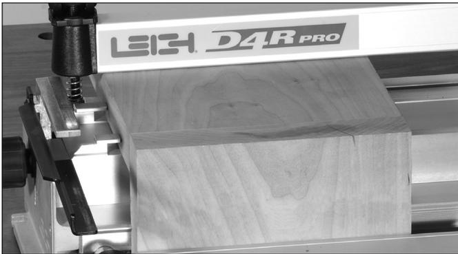
**3** Mount a tail board, **minimum 1/2" thick**, in the front of the jig and be sure to use a backer board mounted horizontally, butting up against the back of the tail board. The backer board should be at least as thick as the depth of cut.
