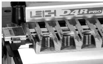
Adjust the depth of cut for perfect joint fit.
