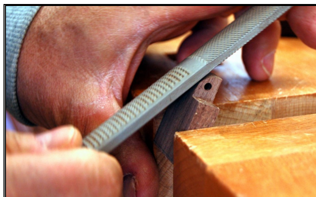
Fine-tuning curvature, to provide turning clearance.
