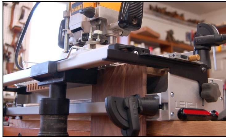
Setup to cut finger joints – these will become wooden hinges.
