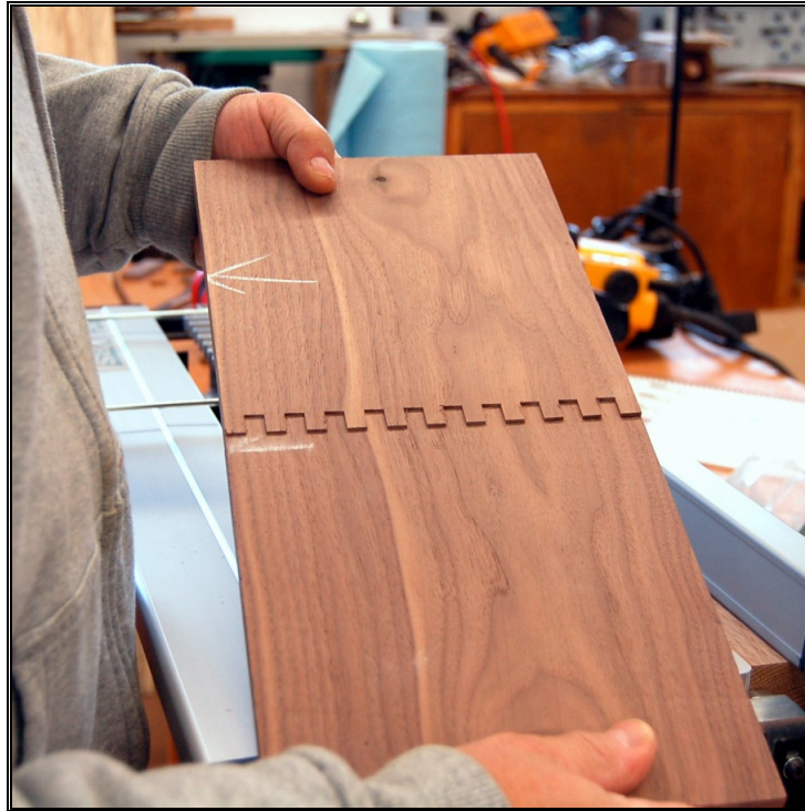
Dialed in the fit - it is 0.004" loose, and perfect.
