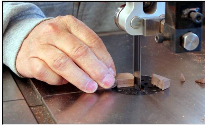
Trimming to rough shape.
