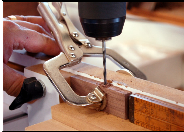
Drilling for hinge pins.
