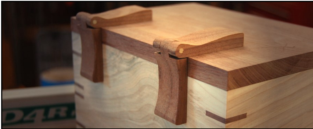
The prototype rounded hinges, as I tried a dry-fit on a box. A little refinement, and it will be ready.
