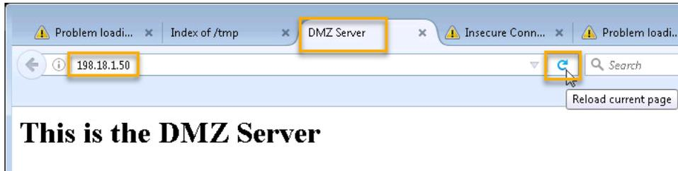
30. On that same workstation open up **FileZilla** and use the **Quickconnect** fields to FTP to the DMZ server's internal IP address (**172.16.102.50**) and log in as **user/C1sco12345**. Don't use the saved link for the DMZ server because it used the DMZ server's outside IP address (198.18.1.50).
