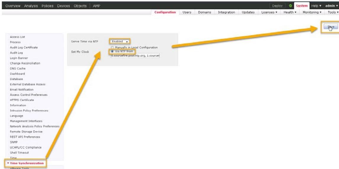
17. Once the page has refreshed go back to the **Time** menu tab again and ensure the time is close to the same time as what is on hq-wkst. (Since the hq-ftd device is not yet configured the NTP service can't update so the time might be a little off until you get through Scenario 3.)
